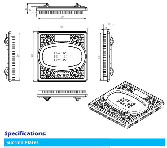
Suction Plate 300 with SMART CUT foam seal
